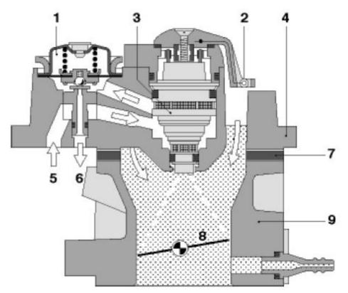
Figure 6: Mono-Jetronic central injection unit
