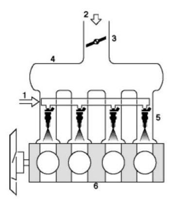
**Figure 8:** Multipoint fuel injection system 1 Fuel, 2 Air, 3 Throttle valve, 4 Intake manifold, 5 Injectors, 6 Engine.
