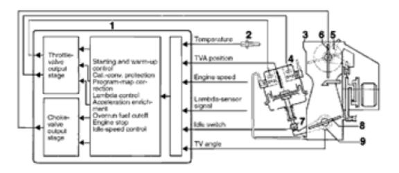
Figure 3: Schematic of an electronically controlled carburettor (ECOTRONIC).
