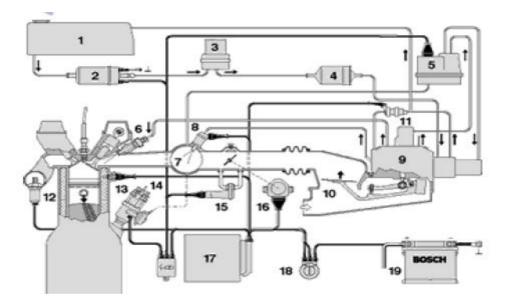
Figure 9: Schematic of a K-Jetronic system
