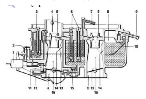
Figure 2: The Schematic of a Two-Stage Carburettor
