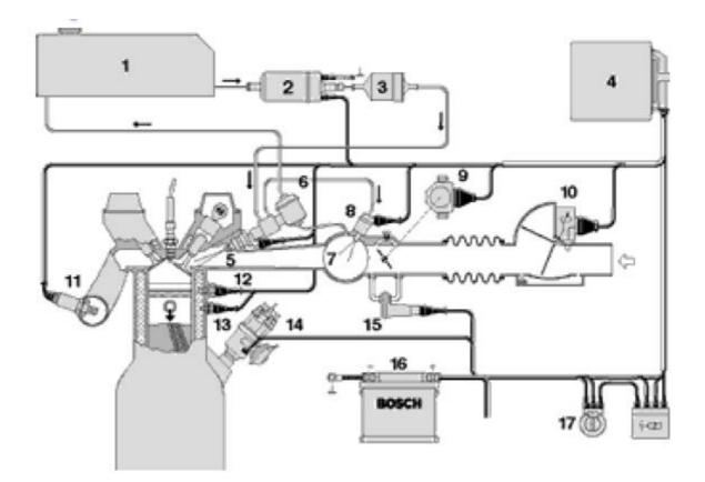
Figure 11: Schematic of an L-Jetronic system
