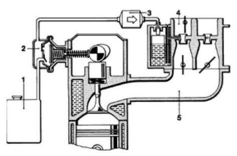
Figure 1: Fuel Metering System
