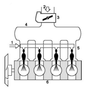
**Figure 6:** Direct injection (DI) system 1 Fuel, 2 Air, 3 Throttle-valve (EGAS), 4 Intake manifold, 5 Injectors, 6 Engine.
