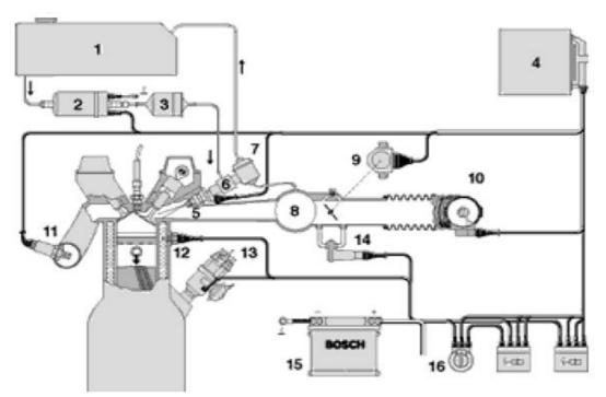
Figure 12: Schematic of an LH-Jetronic system
