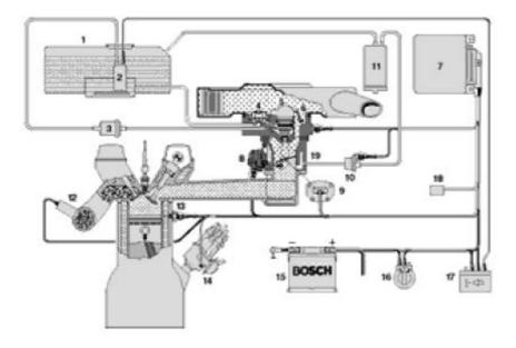
Figure 5: Schematic of a Mono-Jetronic system
