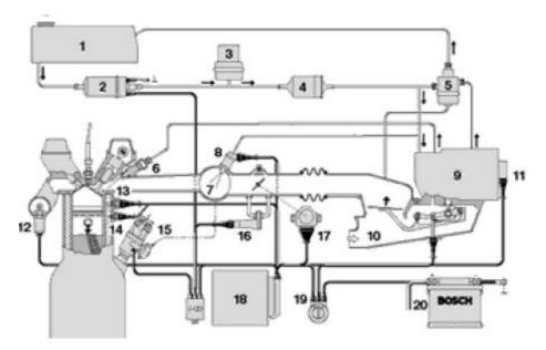
Figure 10: Schematic of a KE-Jetronic system
