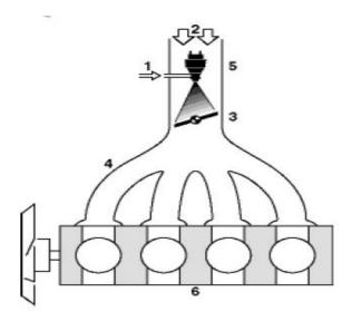
**Figure 4:** Single-point fuel injection system 1 Fuel, 2 Air, 3 Throttle valve, 4 Intake manifold, 5 Injector, 6 Engine.
